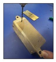
**STEP 2**Drill both holes using a 7/64 drill bit for metal.
