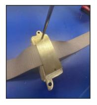
STEP 5 Using a Phillips #2 screw driver, screw the x2 6-32 machine screws, securing the plate the back of the jbox body.
