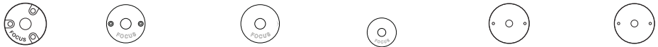
FA24/BRS 3.00" dia. (12v) FA24MDCST/BRS 2.65" dia. (12v) FA24MDCSTPC/BRS 2.65" dia. (12v) FA24MD (12v) FA24LGSPUN/BRS 4.75" dia. (12v) FA24LGCST/BRS 4.75" dia. (12-277v)
