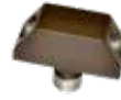
T-Adapter FATAD Size: 3.45" x 3.00" x 1.25" Material: Brass Material Options: Aluminum x2 1/2" NPS Female x 1/2" NPS Male
