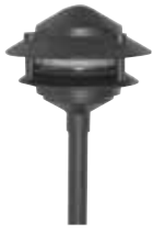
AL03L12BLT (12v) Size: 14.00" x 6.00" dia. Material: Cast Aluminum Material Options: N/A LED: 3w Omni SS LED (L12) CCT: 3000K Lumens: 300lm LED Option: LED Panel (LEDP) ● ALUM
