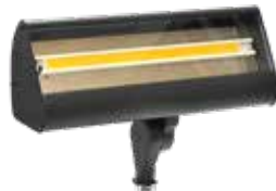
LFL01LED1212VBLT LFL01LED12120VBLT Size: 4.50" x 13.00" x 3.00" Material: Aluminum Material Options: N/A LED: 12w LED Panel CCT: 3000K Lumens: 1080lm CCT/Lumens Option: 52K/1160lm ● ALUM
