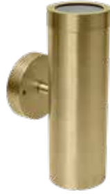
SL16PAR30L154BRS Size: 13.00" x 4.50" dia. Material: Brass Material Options: Aluminum LED: x2 10w PAR30 SS LED 36° (L154) CCT: 3000K Lumens: 1000lm ● ALUM ● BRS
