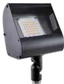
DL10LEDM3030MVBTL (120v/277v) Size: 9.00" x 5.10" x 3.00" Material: Aluminum Material Options: N/A LED: 30w LED Module CCT: 3000K Lumens: 3000lm LED Option: LED Panel CCT Option: 2700K/4100K ● ALUM ● BRS
