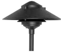
AL0310L12BLT (12v) Size: 14.25" x 10.00" dia. Material: Cast Aluminum Material Options: N/A LED: 3w Omni SS LED (L12) CCT: 3000K Lumens: 300lm LED Option: LED Panel (LEDP) ● ALUM
