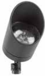
DL42LEDM740BLT Size: 4.50" x 3.125" dia. Material: Aluminum Material Options: Brass LED: 7w LED Module 40° CCT: 2800K Lumens: 450lm Optic Options: 15°/40°/60° WF No Optics ● ALUM ● BRS
