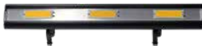
LFL013LEDP812VBLT LFL013LEDP8120VBLT Size: 8.13" x 4.50" dia. Material: Aluminum Material Options: N/A LED: x3 8w LED Panel CCT: 3000K Lumens: 1890lm CCT/Lumens Option: 52K/2040lm ● ALUM
