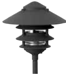
AL034T10L12BLT (12v) Size: 17.75" x 10.00" dia. Material: Cast Aluminum Material Options: N/A LED: 3w Omni SS LED (L12) CCT: 3000K Lumens: 300lm LED Option: LED Panel (LEDP) ● ALUM
