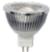
(FLEDMR16SS5W) 5W MR16, GU5.3 BI-PIN BASE, (L34) 15°, (L36) 36°, (L38) 80° 450 LUMEN, 3000K, 40,000 HR
