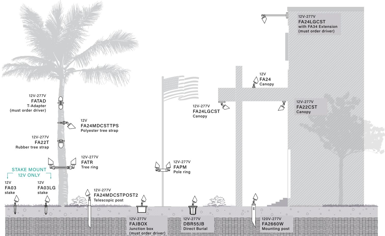
Images enhanced to illustrate usage of mounting options. Drawings not to scale. (see page 2 for product dimensions)
