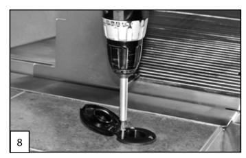
(8) Reuse the three #6 X 1" set up screws to mount Quick Connect Base into mounting sleeve.
