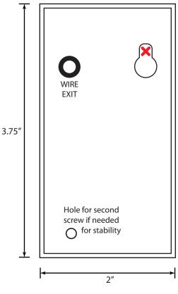
"X" inside key hole marks location of mounting screw
