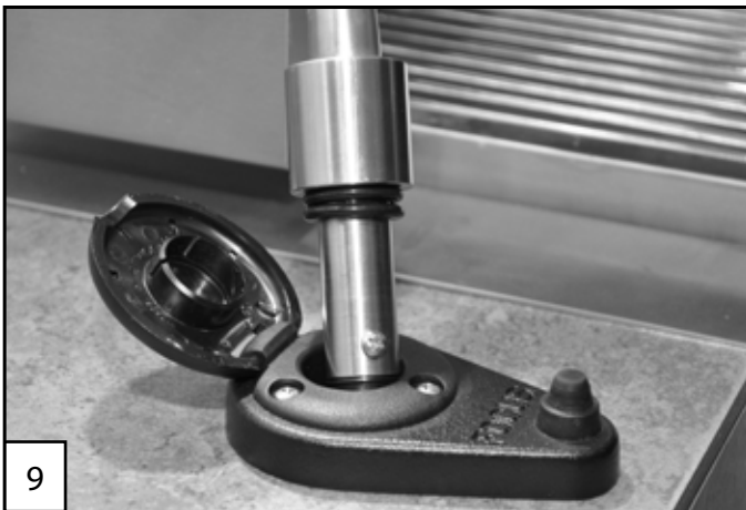
(9) Insert Quick Connect BBQ fixture into base with set screw facing towards front of counter. Press fixture firmly into place. Turn on power and check for proper operation.
