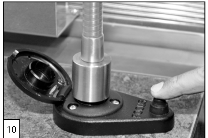
(10) When fixture is in use, the On/Off switch can be used to turn off light without removing fixture. When not in use, pull fixture straight out of base and close cover. Fixture should be stored in a dry area.
